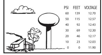
deplete the water supply at an ever decreasing pressure. Although a 12 volt battery is not physically shaped like a water tower, it has most of its stored electricity available between 12 volts to 12.7 volts. When drained below 12 volts, little amperage remains and the battery voltage will decrease rapidly.
