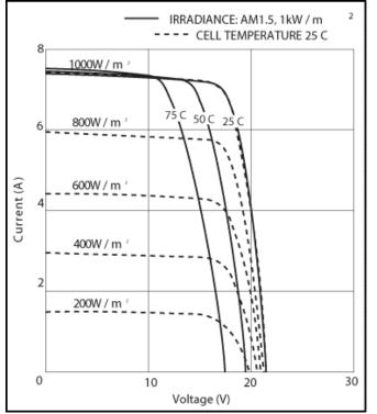
Maximum power is derived at the knee of the curve. Check the amperage generated by the solar array at your battery's present operating voltage to better calculate the actual power developed at your voltages and temperatures.
