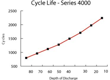
Now what if we used a 110ah battery? We normally recommend that a battery system be sized for no less than 50% depth of discharge. Clients always use more power than they anticipate, so it is a good idea to add a cushion to your calculations. And with solar systems, a planned 20-30% depth of discharge leaves you a few days of safety (autonomy) in case of heavy cloud cover for a few days.
