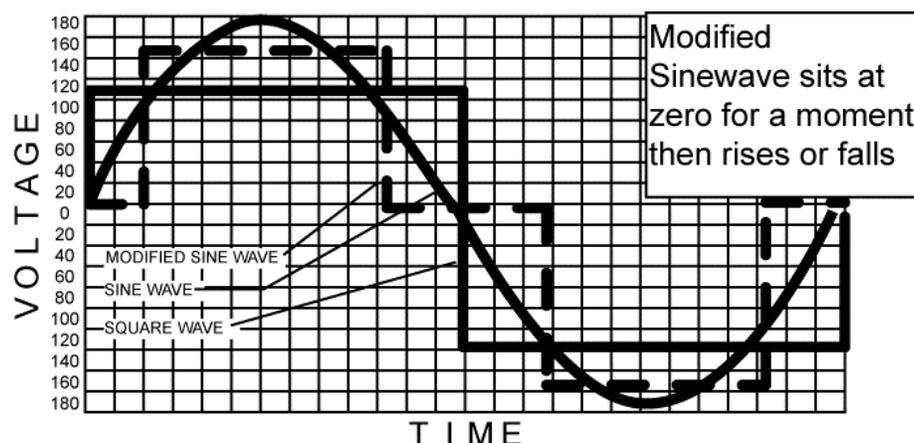
The sine wave smoothly increases to its peak and smoothly decreases in a perfect S shape. Modified sine waves and square waves shoot straight up, level off at peak voltage, and then drop straight down as the current changes directions. The modified sine wave also sits at zero (neutral) for a short period, giving an extra step. This is the main difference between it and the square wave.
