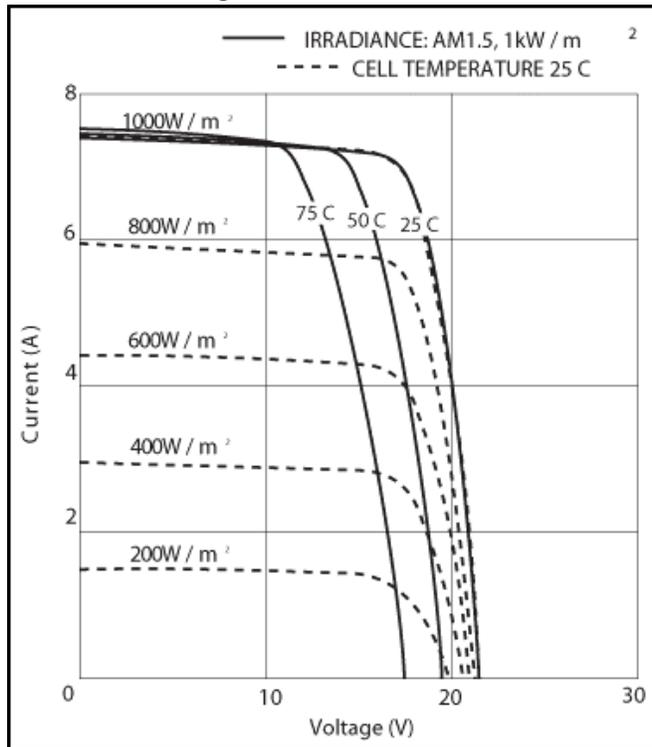
Maximum power is derived at the knee of the curve. Check the amperage generated by the solar array at your battery's present operating voltage to better calculate the actual power developed at your voltages and temperatures.
