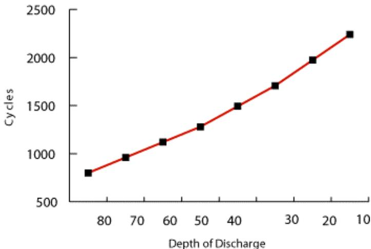
Now what if we used a 110ah battery? We normally recommend that a battery system be sized for no less than 50% depth of discharge. Clients always use more power than they anticipate, so it is a good idea to add a cushion to your calculations. And with solar systems, a planned 20-30% depth of discharge leaves you a few days of safety (autonomy) in case of heavy cloud cover for a few days.
