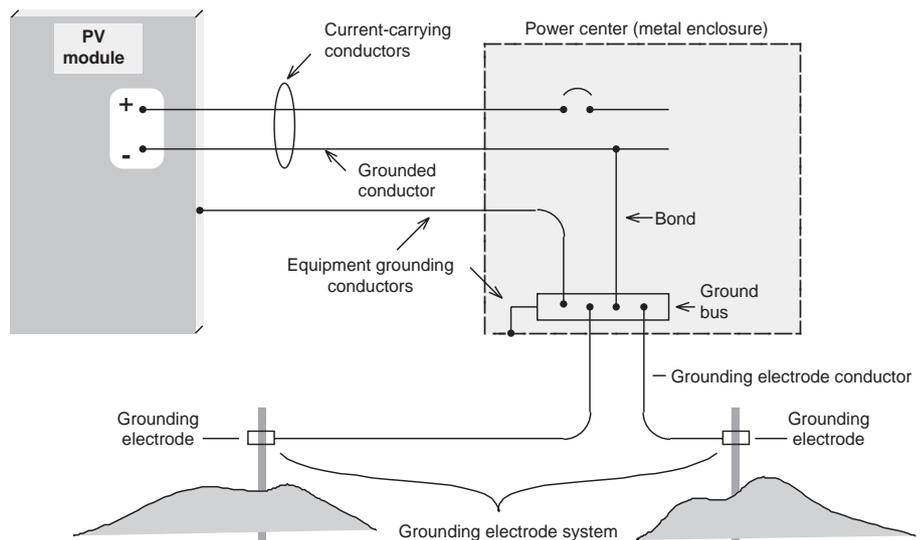
may be bare (uninsulated) or covered with green insulation. They are normally routed along with the current-carrying conductors.
